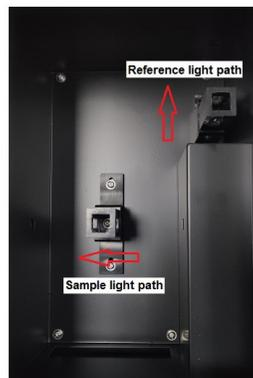
The schematic diagram of the instrument's internal structure is shown in Fig. 1-4:
