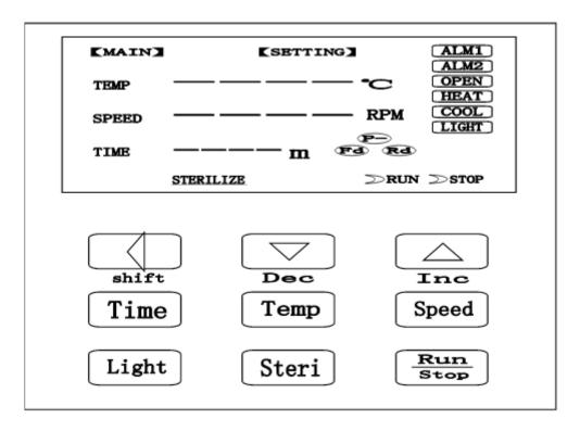
(1) Controller is powered on, the temperature display window showing "HY - 2", speed display window showing "8888", the time display window showing "8888", all identifiers is lighting, the machine into the normal display status after 4 seconds.
