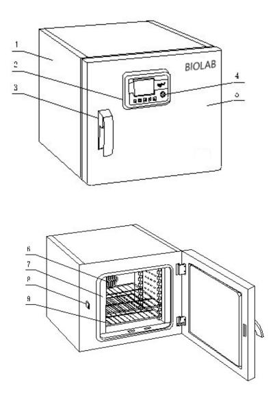
incubator body 2. controller 3.door handle 4. power supply 5.outer door
