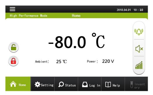
**Home page middle area:** The center of the home page shows inner temperature, the lower left shows ambient temperature, the lower right shows current power voltage, the upper-left corner shows the system working mode (high-performance or energy-saving), the upper-right corner shows system time.
