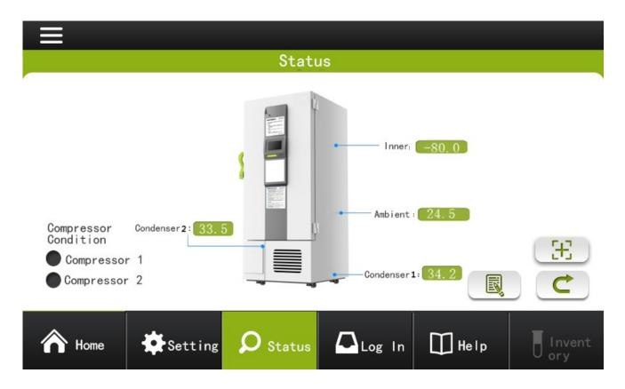
**Compressor status:** The compressor icon is green when the compressor running; the compressor icon is gray when the compressor stops
