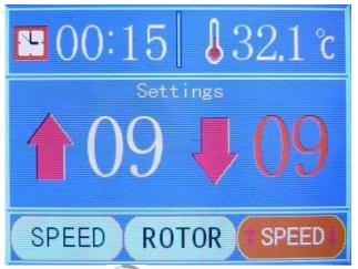
② Press the " UP" button to adjust the acceleration of the rotating speed, or touch the screen and click the icon to do the same operation. There are 10 acceleration levels: 0 is the slowest while 9 is the fastest.
