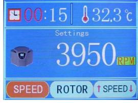
3) On the bottom of the first adjustment panel, press the "SET" SET" button to enter the second adjustment panel (the adjustment panel of rotor modes), or touch the screen and click the rotor number area to enter the same panel. As it is shown below:
