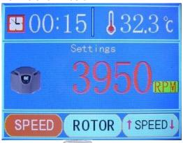
②Press the " SET" button to enter the rotating speed adjustment panel. Next, press the
