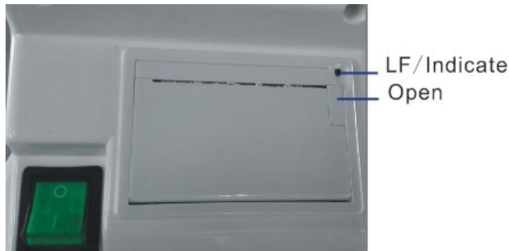
pull “open” button of the printer to open the door,
