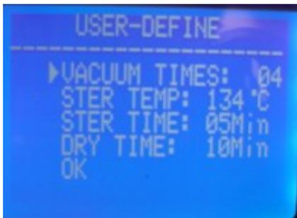
When the cursor is before this option, User can press "UP" or "DOWN" to change the setting.
