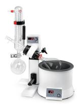
5L heating bath with a wide temperature range (room temp. to 180°C). Independent temperature control makes it can be used separately. Water/oil heating mode can be changed just through a switch
