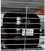
Without fluorine R134a refrigeration compressor
