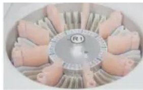
Reagent Tray 2~8°C cooling for 24 hours.
