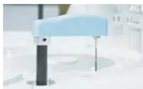
Reagent Tray 2~8°C cooling for 24 hours.
