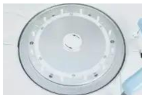
Reaction Tray 37±0.1°C, real-time monitor.
