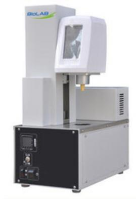
One-click automatic lifting structure. Software can calibrate viscometer and analyze linear accuracy. Can test after 2 hours constant temperature with the efficiency almost increased 90%
