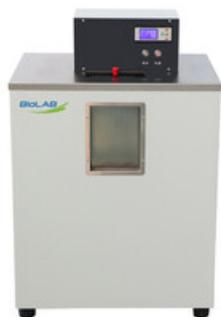
The temperature of the constant temperature bath is controlled by the temperature controller, and the refrigeration and heating parts compensate each other to achieve heat balance and maintain a certain accuracy in controlling the bath temperature. The instrument can install two samples for test at the same time. The constant temperature bath is equipped with a stirring motor to make the temperature in the whole constant temperature bath uniform.
