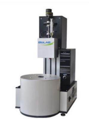
Automatically calculate calibration error of standard oil. Viscosity measuring range:1500-25000cp. Check the accuracy of data for users. Can edit dozens of standard oil.
