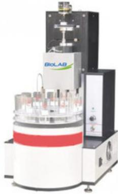
Automatically calculate calibration error of standard oil. Viscosity measuring range:1500-25000cp. Check the accuracy of data for users. Can edit dozens of standard oil. Test component of -40°C is optional.
