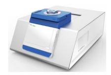
Four channel fluorescent detection system with LED light source and high resolution CCD
