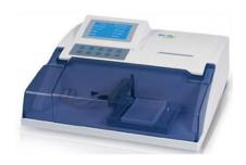
User friendly operation system with large LCD display. Washes flat, U and V-bottom strips and plate.
