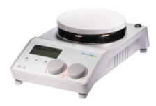
External temperature sensor PT1000 is available for hotplate model, real-time controls medium temperature.
