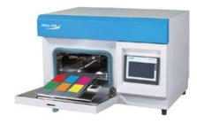
The xenon arc lamp reoccurs the full solar spectrum vividly which include ultraviolet, visible light and red light.
