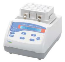
Optimized 2D mixing designed for simultaneous mixing and vortexing applications Pre-programmed soft keys and reliable universal holder Automatic imbalance detection and anti-spill technology Mixing in a 3-in-1 format: Plates (up to 96-well and 384-well formats),Micro-Tubes, Vortexing numerous tube formats Custom blocks available for different experiment needs
