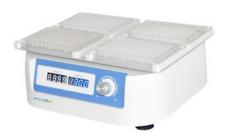
Variable speed from 200 rpm to 1,500 rpm
