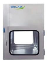
Photoelectric sensor, automatic blowing Adapt with circulation wind to ensure the cleanness of shower area under non-shower status Double door by electric interlock LED display with adjustable blowing time(0-99s) HEPA filter, Class 100 cleanness
