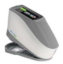
45/0 geometrical optics structure, comply with CIE, the testing conditions of MO, M 1, M2, M3 stipulated by ISO 13655 standard, it can accurately measure various printing density, overprint rate and other printing parameters.
