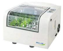
PID controller Forced convection circulation Stainless steel internal material Audio and visual alarm for over-temperature Alarm: Over-speeds, Independent over-temperature protector, Shutdown protection for door opening, Leakage or over-current protection. Optional accessories: UV lamp, humidity controller, inlet air pipe, light system, etc.
