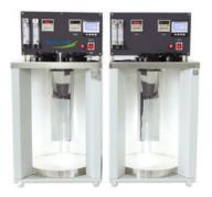
The instrument is used to determine the foaming tendency and stability of lubricating oils. he instrument adopts all-in-one structure. It includes three parts: low temperature test part and it's control, high temperature test part and it's control, a portable cooler for low temperature test part. The instrument equips an automatic timing alarm.
