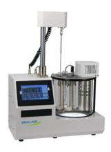
The instrument is suitable to determine the water separability of petroleum oils and synthetic fluids. It adopts LCD to show the diagram. Intuitive and clear. Man-machine dialog. Menu type input. Easy to use.
