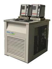
Dry type over speed refrigeration technology without medium. Temperature of two troughs are controlled separately. Compact structure, can put on platform directly
