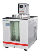
Low noise magnetic pump cross circulation structure. Can test density of antifreeze
