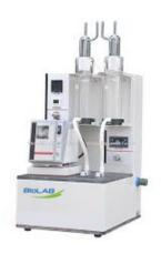
Temperature of bath and air are controlled separately. Automatically control blowing time and defoaming time, accuracy can reach 0.01s. Press-on joint is easy to dismantle tube.
