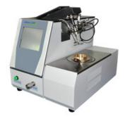
Automatic forced air cooling after test. Flame size is adjustable. Protect program and self-diagnosis function.
