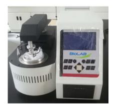
Adopt split structure. Automatical correct influence of atmospheric pressure, and calculate corrected value. Automatic forced air cooling after test.
