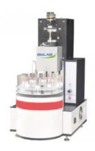
Automatically calculate calibration error of standard oil. Viscosity measuring range:1500-25000cp. Check the accuracy of data for users. Can edit dozens of standard oil. Test component of -40°C is optional.
