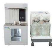
It adopts micro-controller control technology, program control, automatic washing. It needs less solvent oil and it is convenient, efficient. It can be widely used in the enterprises producing and using petroleum products, colleges and universities, and scientific research institutes and so on, where capillary viscometer are used. High degree automation.
