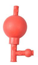
Our pinch and release valve system allows for one-hand operation
