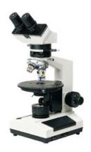
The model has a sliding trinocular viewing head at 45° which is 360° rotatable. Valid mould proof design. It can be used under the high temperature and high humidity environment.
