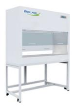
Microprocessor controller Double side work bench, operators can sit face to face Pre-filter: Polyester fiber, washable UV lamp: Emission of 253.7 nanometers
