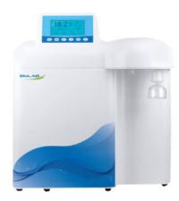
With tap water inlet, to produce RO water and ultrapure water, quality can reach to 18.2 MO.cm.
