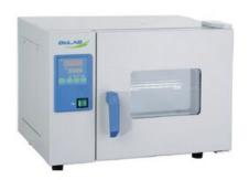
P.I.D temperature controller provides accurate and reliable temperature control
