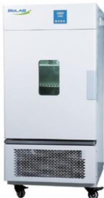
Polished stainless-steel chamber, semicircular arcs at corners for easy cleaning, and the space between the shelves in the chamber is adjustable
