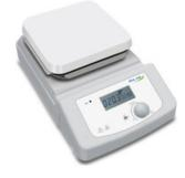
Max. heating temperature is 380°C High resolution LCD displays actual temperature Aluminum cover with ceramic work plate, allows for immediate heat transfer External temperature control is possible with temperature sensor PT1000 Digital temperature control with max. temperature at 380°C
