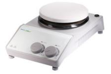
Stainless steel with ceramic coated hotplate resists to corrosion Separated safety circuit, automatically stop heating when temperature over 350°C Motor with electronic speed control, constant speed even during changes in load Variable speed of motor High magnetic adhesion, prevent the stirrer bar escape
