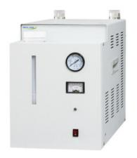
Automatic control, constant pressure, constant flow Ultra high molecular membrane separation technique, PCAN carrier and precious metal catalyst Deoxidation and Dehydration device, high purity Compact, frees up valuable space Easy operation, meliminate the need for expensive gas cylinder Safe and reliable
