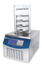
Condenser, control panel, shelves and trays are made of stainless steel Low noise compressor with a long shelf life The drying chamber is equipped with organic glass for safety and visibility Condenser features pre-freezing function Features vacuum freeze drying technology Drying curves are displayed on LCD screen Tray spacing can be customized Eco-friendly CFC free refrigeration system Features nitrogen valve and eutectic test device (optional)
