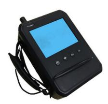
High accurate and flexible identification of a wide range of the unknown substance with extensible substance library
