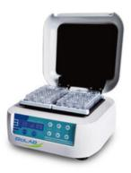
LCD display. Setting temperature and actual temperature simultaneously displayed. Diminishing time displayed.
