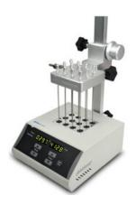
The height of the air chamber plate can be adjusted. The length of a standard gas needle is  $150\ \text{mm}$
