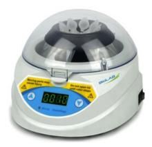
Large radius rotor with 8 tube holes, centrifugal force is 1.7times bigger than ordinary 6-hole rotor
