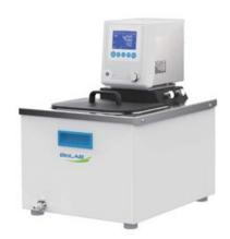
Microprocessor temperature controller with LCD screen ensures precise and reliable control, easy to operate
