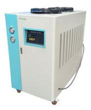
It adopts single-stage vapor compression circuit and has compressor overload protection, pump overload protection, reverse phase and lack of phase warning, antiicing protection, high and low pressure protection and other devices.
