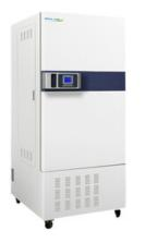
Forced convection mode 30 Stages programmable Micocomputer PID Imported environmental protection insulation materials Excellent Imported temperature and humidity Sensor SUS304 stainless steel interior material ALLCOLDTM: Refrigeration Technology ALLIGENTTM: Humidification System ALLFLOWTM: Perfect Air Current Cycling
