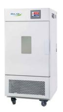
Polished stainless-steel chamber, semicircular arcs at corners for easy cleaning, and the height between the shelves in the chamber are adjustable
