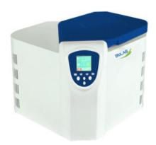
Microcomputer controlled programmable operation with push-button operation
