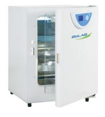
LCD screen, micro computer PID control that can display temp. CO2 concentration, related humidity, operation failure reminder and menu operation are easily to observe and use
