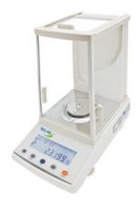
Electromagnetic balanced sensors
