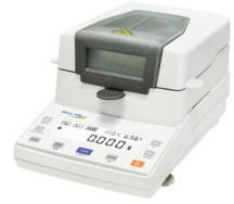
Halogen Light Heating Stainless Steel Chamber Temperature and time can be set The percentage of moisture content The perc entage of dry residual The super high resolution back window matrix liquid crystal display (LCD), making it easier to operate in the dark place, and the user will have a more comfortable vision.
